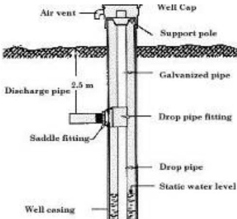
Wells with pitless units have the casing extending up above the ground surface. Wells which have pitless adapter units have a cap that sits down over the well casing (sometimes they have three little set screws on the side of the cap to secure it).
